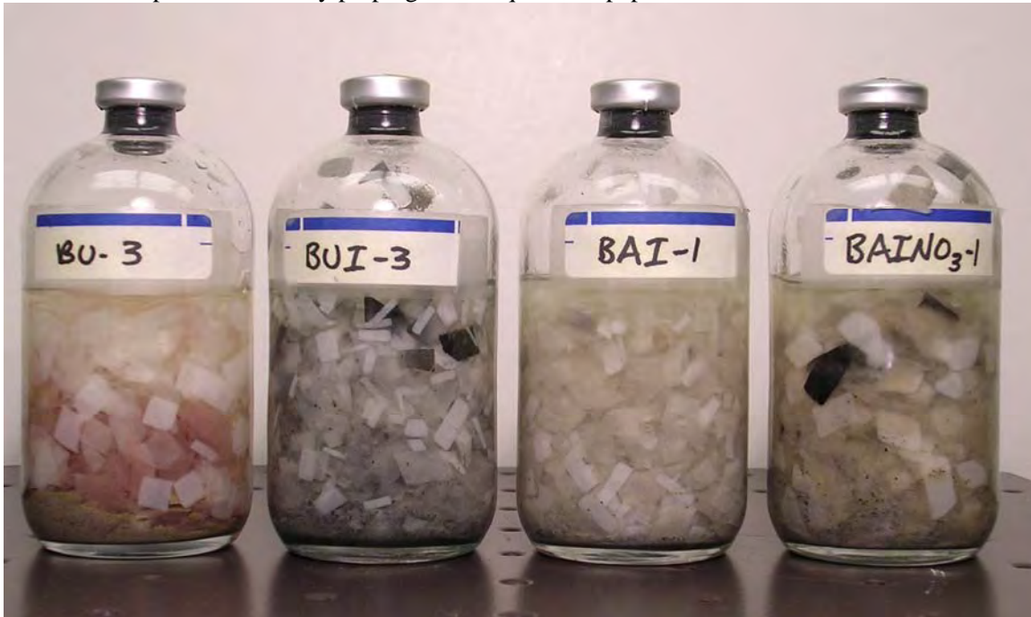
Figure 5(b). Photograph of aerobic samples with bentonite at 3929 days (10.8 years) incubation: unamended uninoculated (BU-3), unamended inoculated (BUI-3), amended inoculated (BAI-1), and amended inoculated plus excess nitrate (BAINO 3 -1). Blackening in BUI-3 and BAINO 3 -1 is due to iron sulfide formation. The brown paper towel in BU-3 is clearly evident while BAI-1 shows loss of color.
