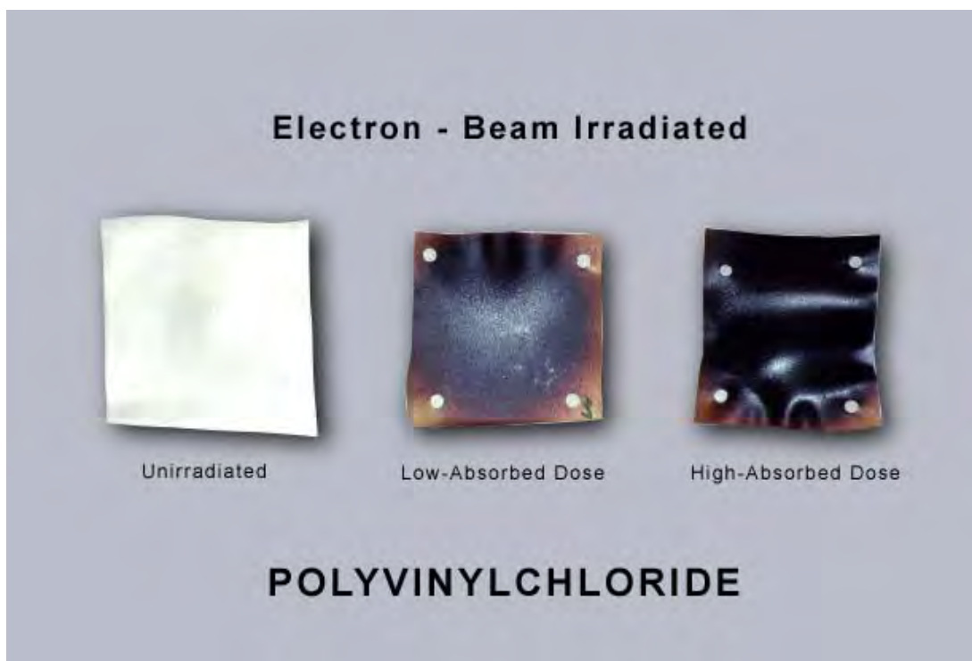
Figure 23. Unirradiated and irradiated (low-absorbed dose, and high-absorbed dose) polyvinylchloride. Radiation caused extreme discoloration and embrittlement.
