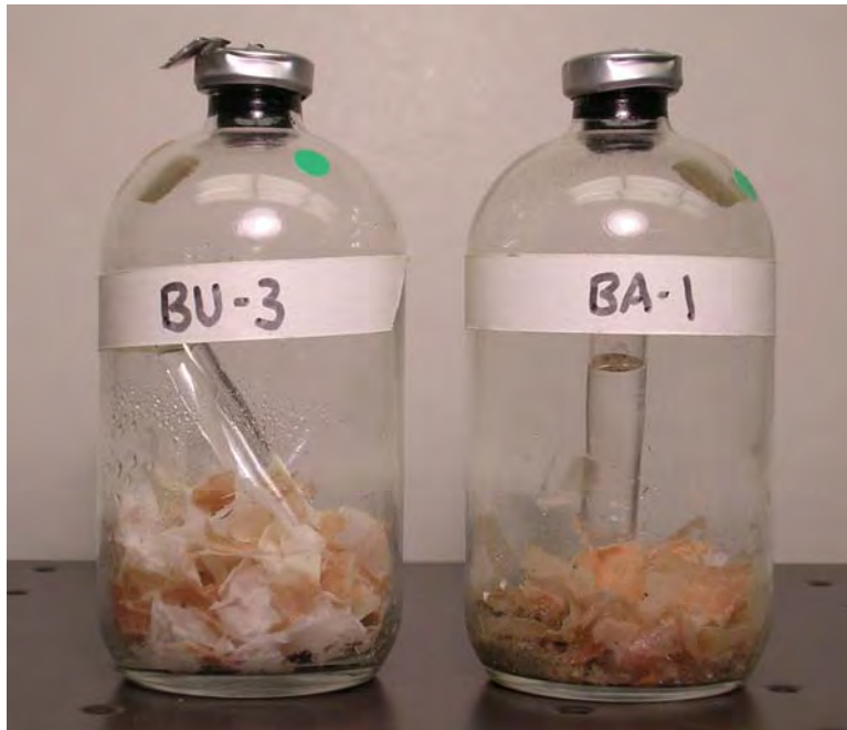
Figure 16(b). Initially aerobic humid samples containing bentonite at 3334 days (9.1 years) incubation : unamended inoculated (BU-3) and amended inoculated (BA-1). The paper in BA-1 has compacted and a biofilm has formed on the paper as indicated by a red color.
